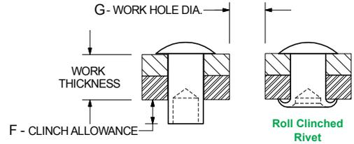
\* LENGTH (in 32nds) = WORK THICKNESS + CLINCH ALLOWANCE "F" (Example Part #: C1-9-ST for 1/8 x 9/32 - specify material and finish)
