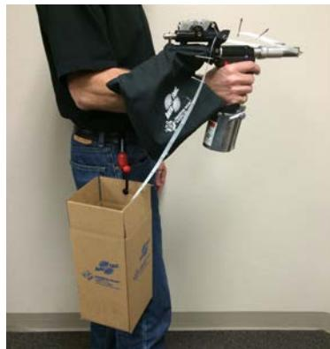
We supply almost any size, type and material of blind rivet loaded on plastic tape ready for the **AutoFast**<sup>®</sup> system. **AutoFast**<sup>®</sup> is up to 4 times faster than hand loading rivets, as fast as 60 rivets per minute!
